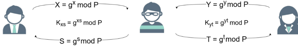
Figure 1. Man-in-the-Middle Attack on Diffie-Hellman Key Exchange Protocol
