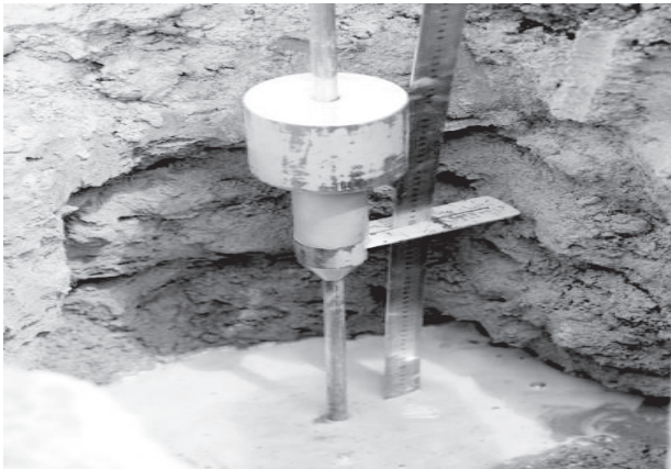
Figure 13. Subgrade layer saturated by water at Ranakharia Mosque
