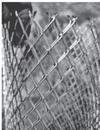
Figure 2. SSWM case preparation: tying with SSW (left), sewing with SSW (right)
