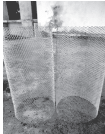
Figure 1. Specimen preparation: unwrapped specimen (left), Stainless-Steel Wire Mesh cases (right)
